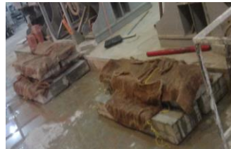
Figure 8: Curing of Tested Beams
