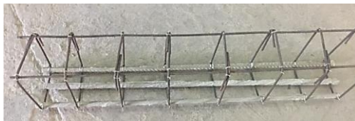
Figure 5: GFRP bars of Some Tested Beams
