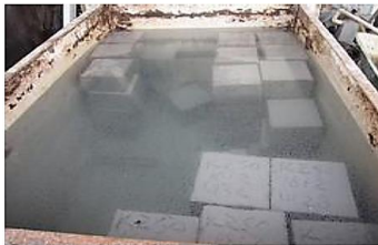
Figure 7: Curing of Concrete Cubes
