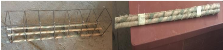
Figure 6: HFRP (Hybrid Fiber Reinforced Polymer) Bars of Some Tested Beams
