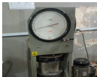
Figure 2: Compression Test of Concrete Cube
