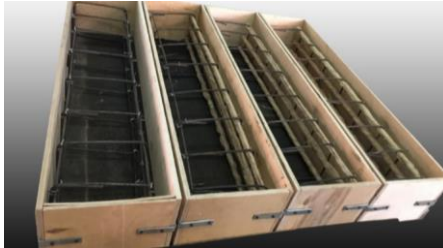
Figure 3: Fiber Reinforcement of Some Tested Beams
